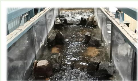
Fig. 3. Physical model of step-pool NLF. A model scale of 1: 4 was chosen. The step-weir arches in the upstream direction. Experiments are conducted at the Hydraulics Laboratory of IIT Madras
