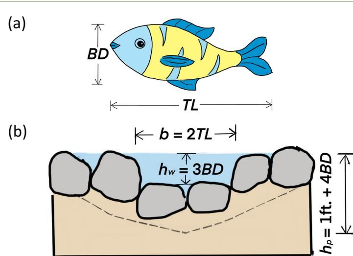
Fig. 2. (a) Body measurements of the largest target species, (b) Weir section of step-pool NLF, where  $b$  = weir opening width,  $h_w$  = weir opening depth,  $h_p$  = pool depth
