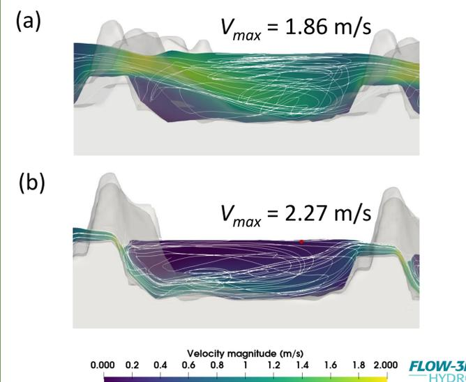
Fig. 4. The contour of velocity magnitude along the centreline of step-pool NLF at  $Q = 0.5 \text{ m}^3/\text{s}$  for  $b/B$ : (a) 0.30, and (b) 0.70. The former provides sufficient flow depth and acceptable velocity ranges.
